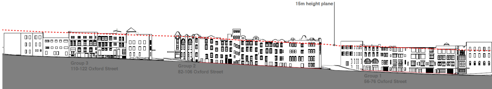
15m height control – Foley Street
