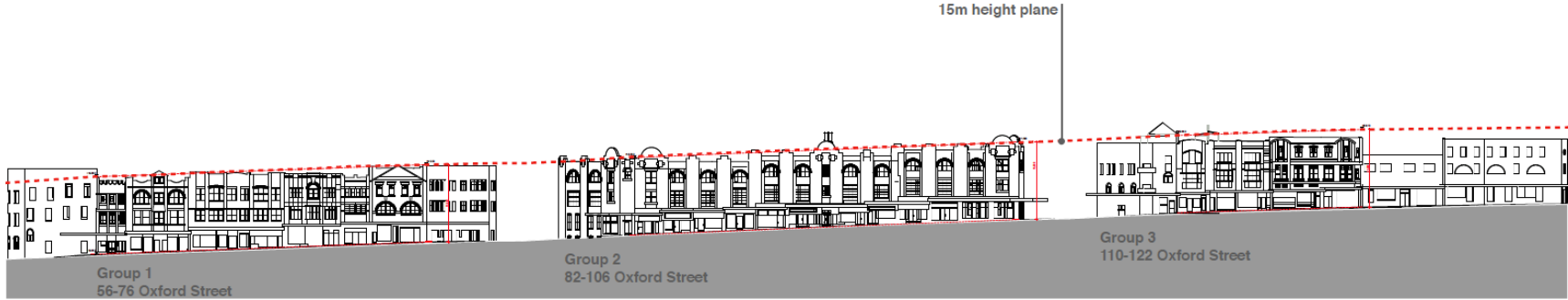
15m height control – Oxford Street
